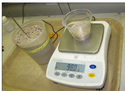
Figure 7: Weighing 98 g of washed sand.
