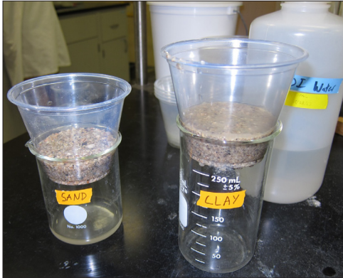
Figure 11: Allowing water to percolate through soil before adding solutions.
