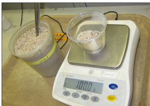
Figure 5: Weighing 100 g of washed sand.
