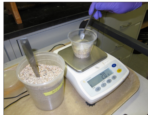
Figure 8: Weighing 2 g of bentonite clay.
