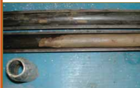
Fig. 2. An opened split spoon with the soil core that has been collected.
