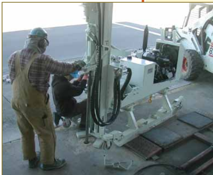
Fig. 1. A skid-mounted direct push probe using a hydraulic percussive hammer and a split spoon.
